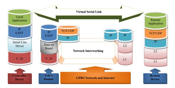
This particular implementation allows to the devices interfacing to the Telit GL865-DUAL/QUAD V3 module the use of the GPRS and Internet packet service without the need to have an internal TCP/IP stack since this function is embedded in the module.
