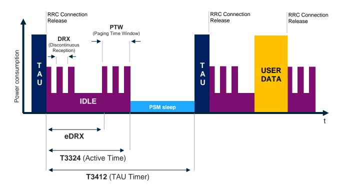
PSM and eDRX are two different features defined in the latest 3GPP releases. The goal of these features is to reduce the power consumption of IoT devices. To achieve this, PSM and eDRX enable different mechanisms to reduce the signalling between the IoT device and network. The picture above shows the two features combined. However, they can be enabled independently.
