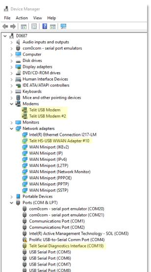
USB Modem ports are ACM devices and can be used as AT Command interface.
