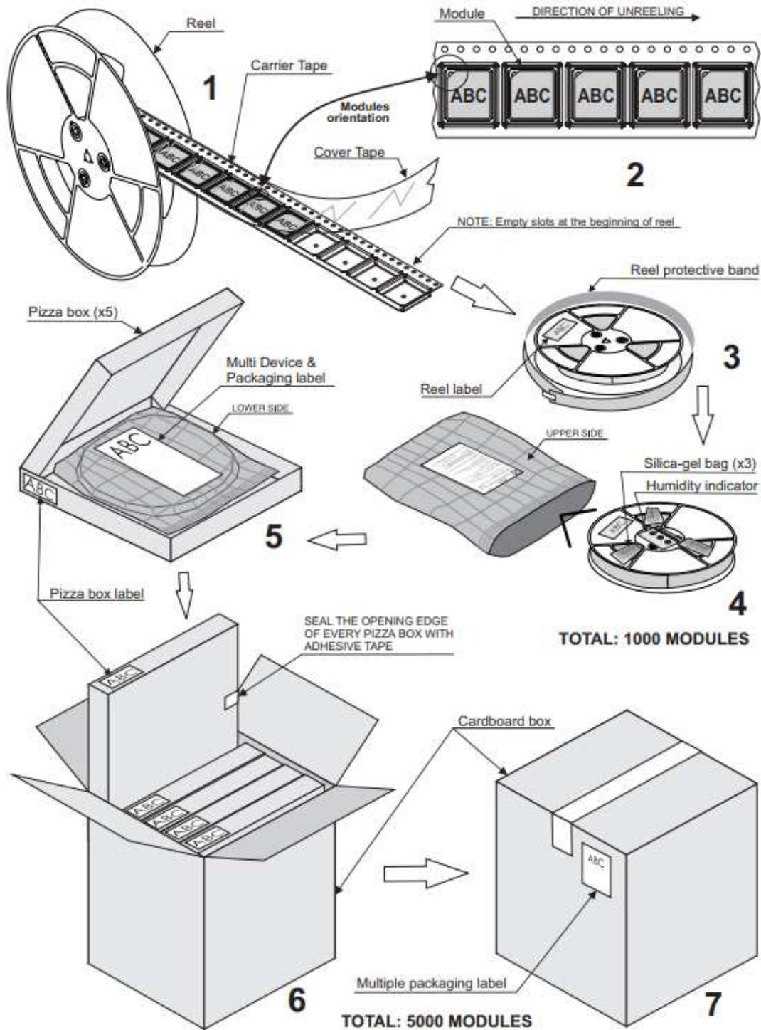
Figure 19: NE310L2-W1 Module Positioning into the Carrier
