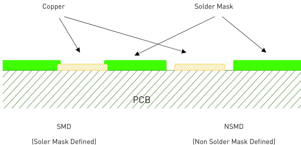
Figure 13: PCB solder pad recommendations
