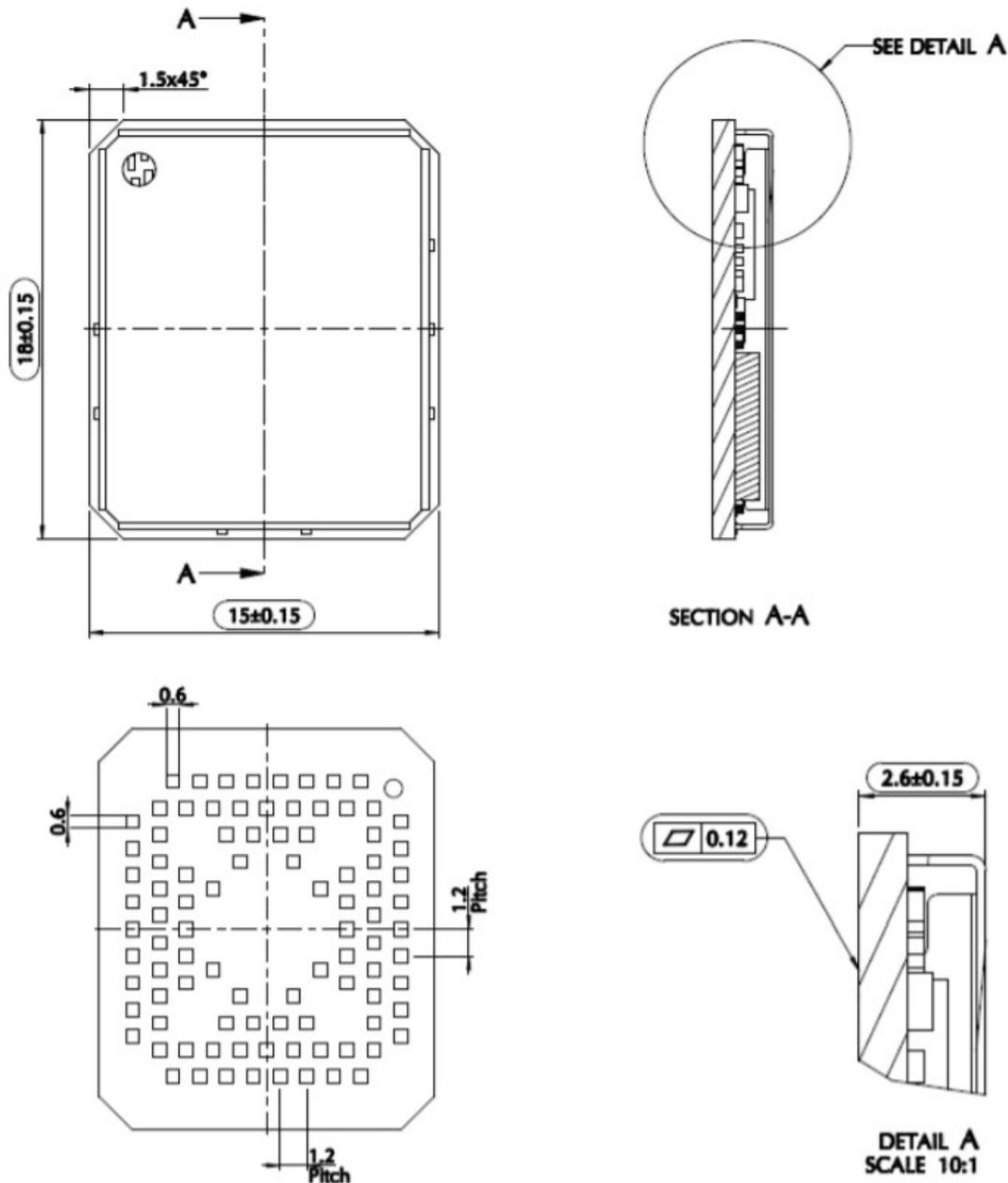
Figure 7: Mechanical Drawing NE310L2-WW
