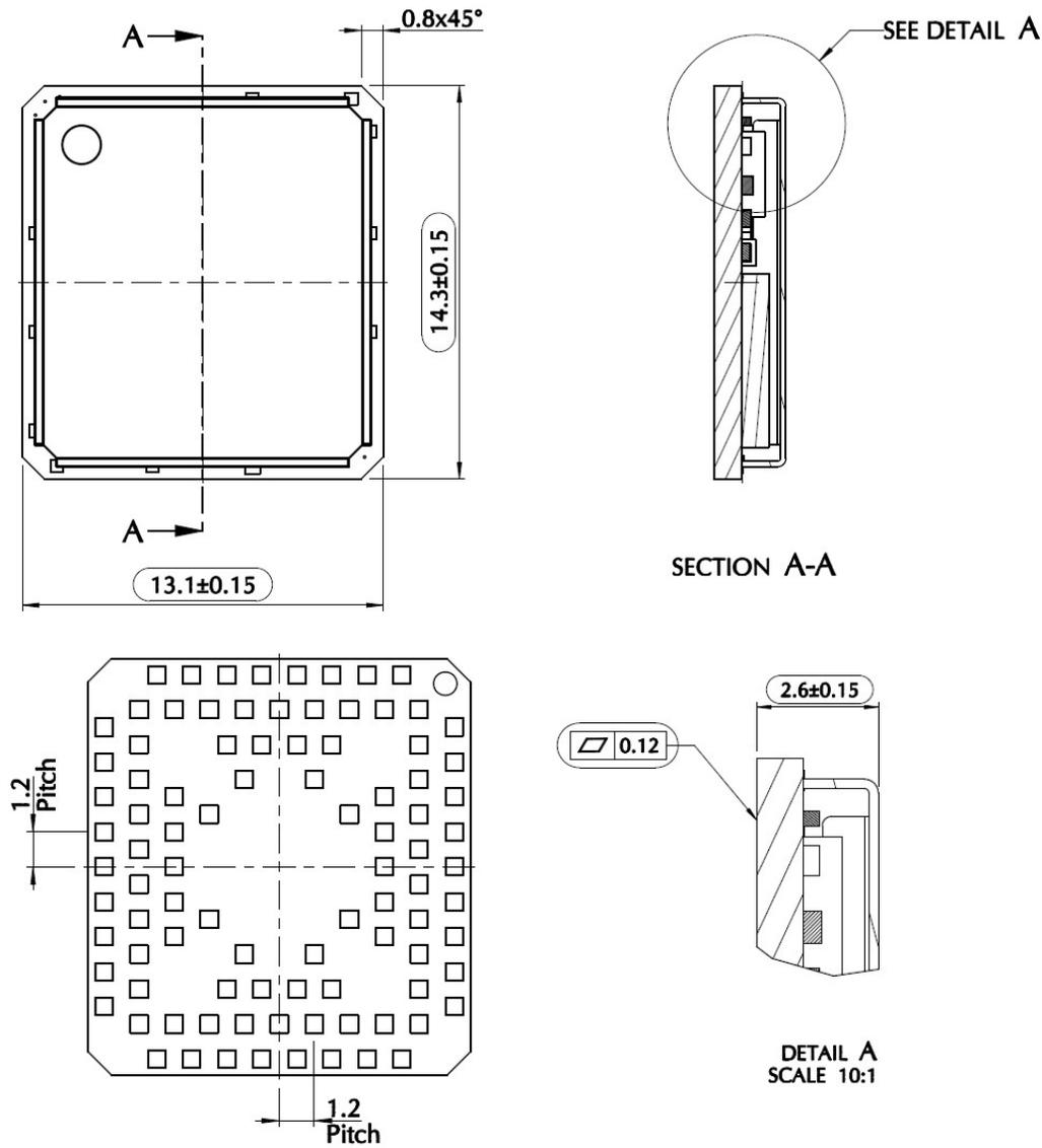
Figure 6: Mechanical Drawing NE310L2-W1
