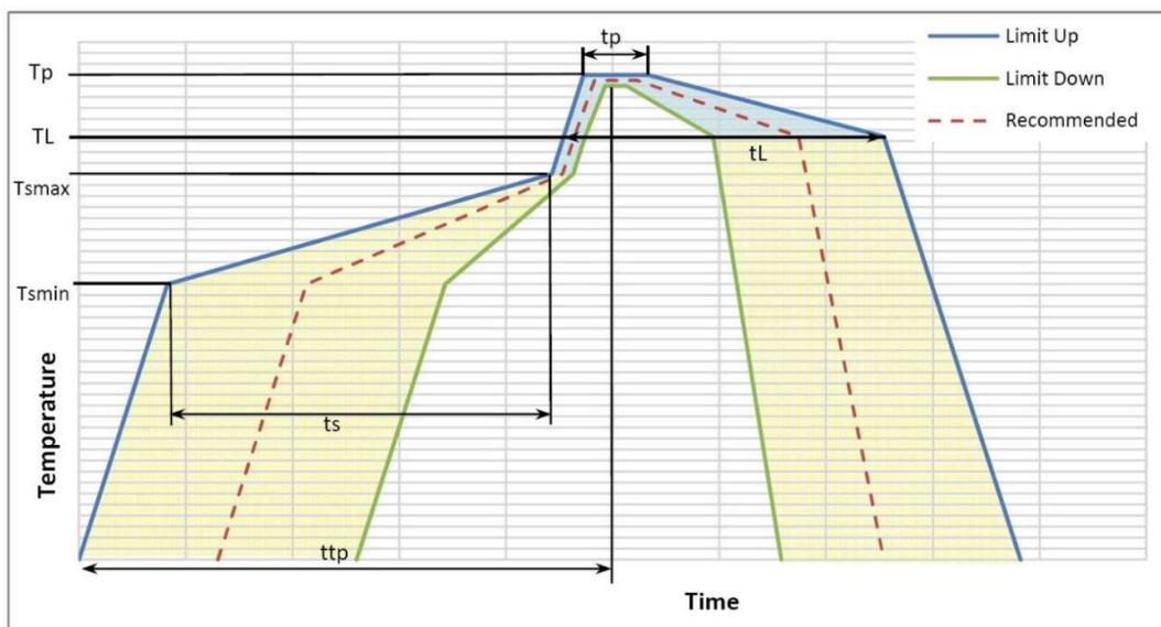
Figure 14: Recommended Solder reflow profile
