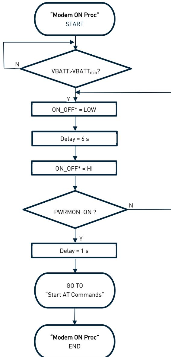
**Note:** Do not use any pull up resistor on the ON\_OFF\* line, it is internally pulled up. Using pull up resistor may bring to latch up problems on the NE310L2 power regulator and improper power on/off of the module. The ON\_OFF\* line must be connected only in open collector or open drain configuration.
