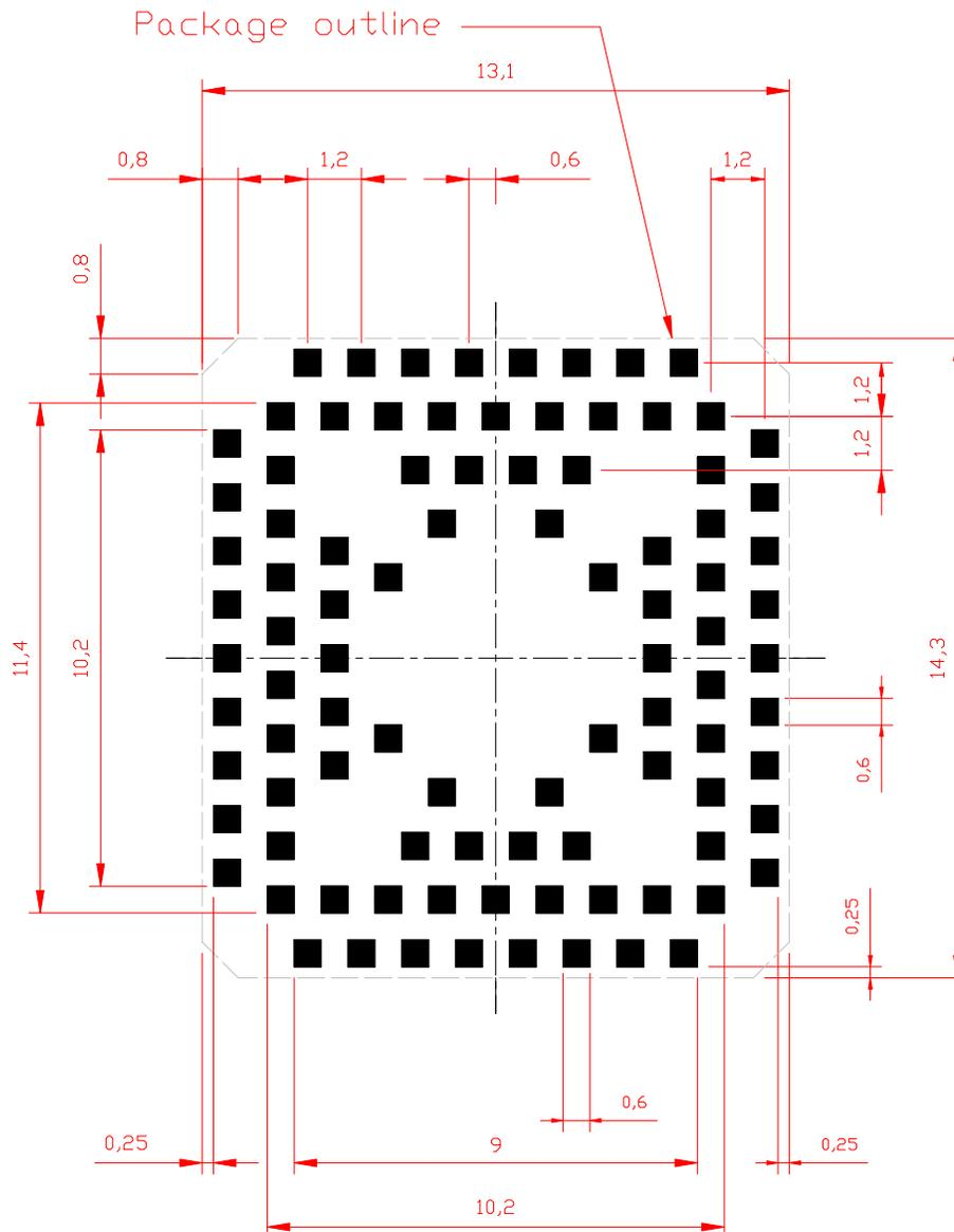
Figure 7: NE310L2-W1 Copper Pattern (top view)
