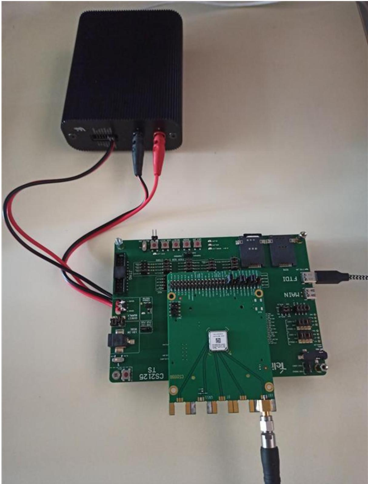
Figure 2: Otii setup with EVB/TLB
