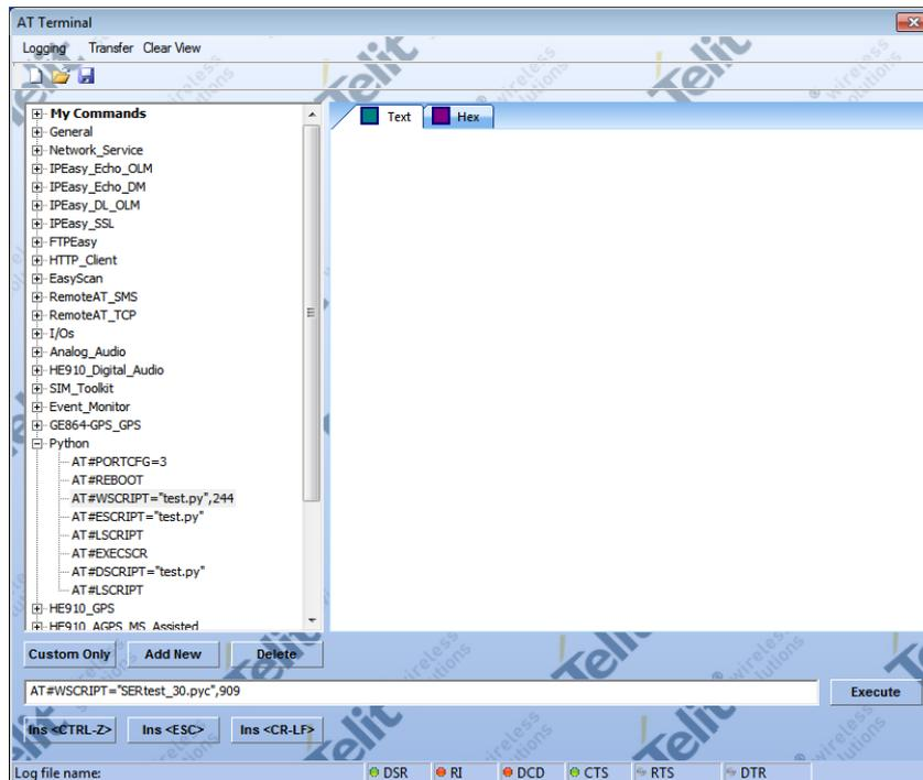
then select the Transfer option to select and transfer the desired file from PC to the module:
