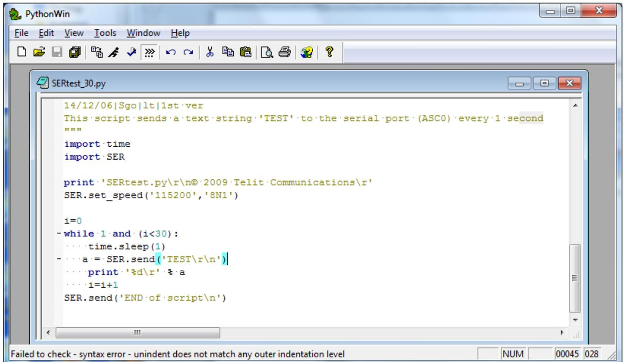
In this picture above, an error is displayed after the “Check” button was pressed. The error is displayed, because “a = SER.send(‘TEST\r\n’)” is not correctly indented. In the bottom picture, the syntax error was corrected and the check operation reports a message “Successful”.
