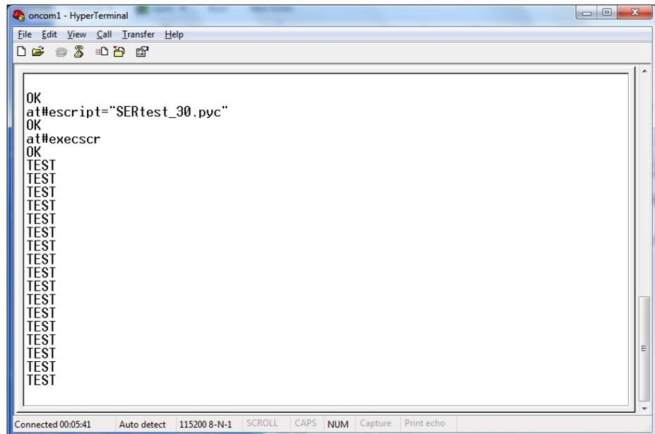
This example should print a series of “TEST” string on the port associated with AT command port (USIF0) and a series of “1” on the debug port (USIF1). The response “1” on debug port is resulting from successful “SER.send” operation.
