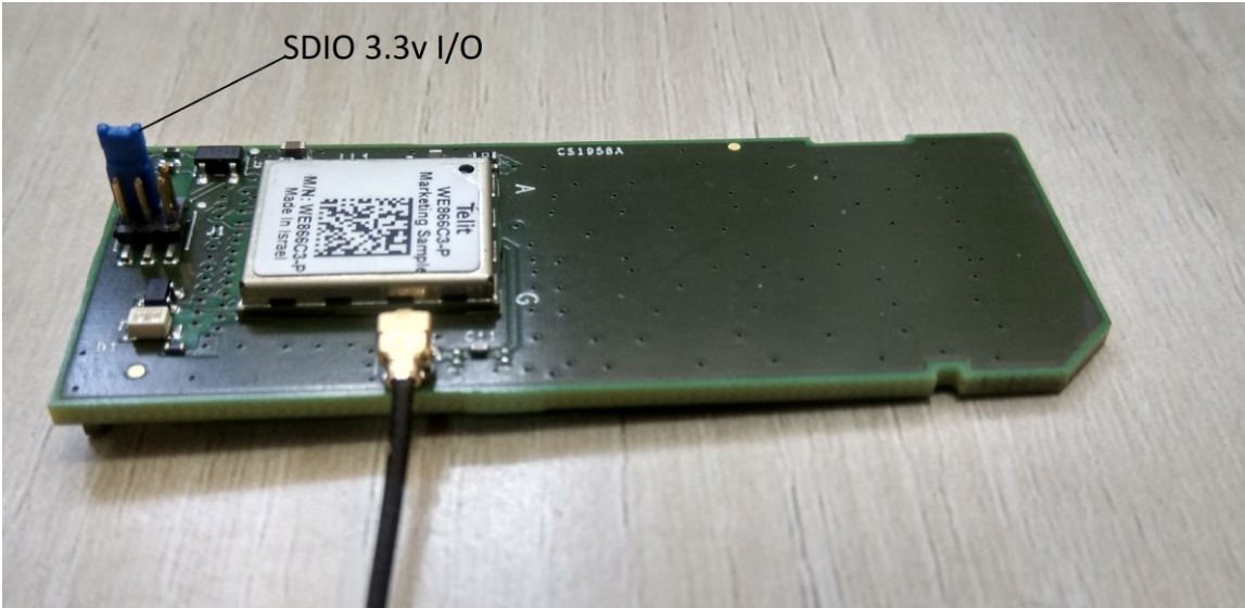
Figure 3-6 Jumper Position for 3.3v SDIO Signal
